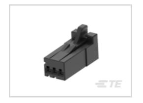
Connector Product Type: Housing Connector & Housing Type: Receptacle Connector System: Wire-to-Board Number of Positions: 3 Centerline (Pitch): 2.5 mm [.098 in ]
