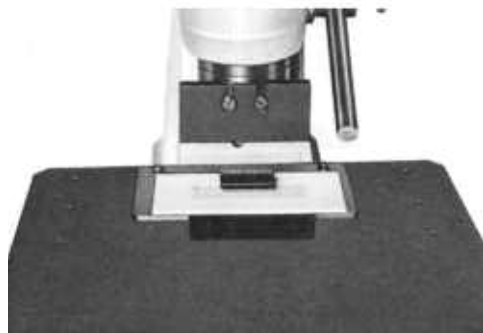
3. Set insertion support plate in place by butting it against Mini-Press platform.
