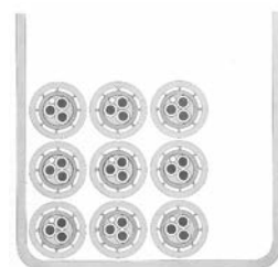
A typical saving in the cable tray volume can exceed 40%
