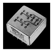
The 4PDT .150 Grid-space hybrid relays are advanced designs of the standard high reliability 4PDT .150 Grid-space relays. In the single diode version, the relay coilback electromotive force is suppressed to prevent circuit/component damage. With the dual diode version, a steering diode is added to the coil circuit, along with the suppression diode. This
