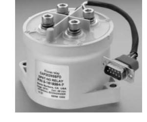
1 Using 4/0 conductor. Current rating is affected by attached conductor size and design. Keep terminals below 150°C max. continuous. 175°C for 2 hours max. and 200°C 270Vdc for 1 minute max. For mounting large conductors, request terminal adapter PN 3-1618396-7. Operational contact resistance is measured by millivolt drop across 270Vdc
