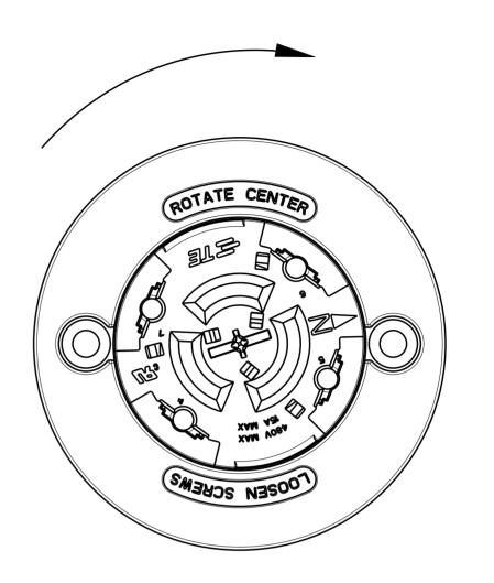
STEP 1: ALIGN THE TE LOGO WITH ONE OF THE SCREW HOLES ON THE LOCK RING.
