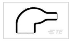
Molded Part Angle: 90 ° Molded Part Shape Code: 222 Lipped: No Material Code: 3 Heat Shrink Boot Material Systems Code: 10
