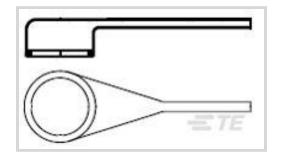
Molded Part Shape: 90° Molded Part Shape Code: 222
