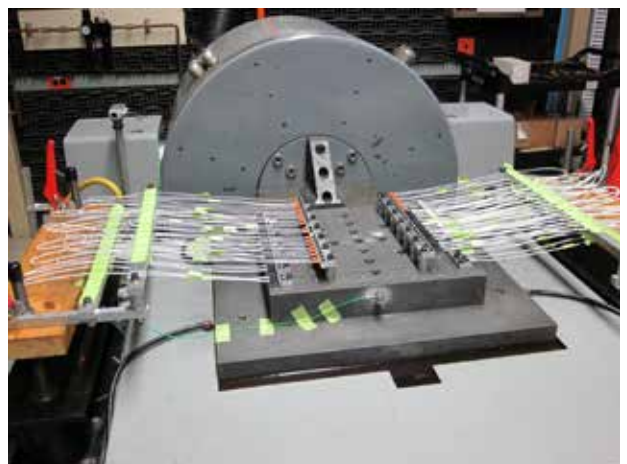
Figure 3 – Military Vibration Test - PIDG Terminals
