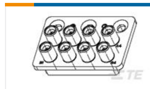
TE Part #1996706-1 8 POS VITA 67.2 RF MODULE, BACKPLANE, SMPM
