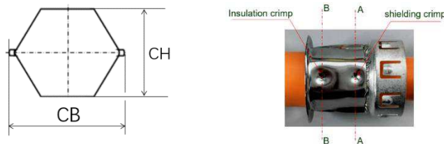
Figure 13: shielding crimp Height and Width
