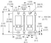
24A110 – Mounting track Mounting track is designed to accept snap-mount sockets, as well as other P&B screw terminal sockets. Track is made of lightweight, sturdy extruded aluminum and is shipped in three-foot (914cm) lengths with mounting holes on six-inch (152mm) centers. Track can be cut to shorter lengths or used end-to-end.
