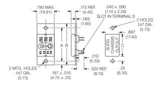
Track mount sockets 27E460, 27E461, 27E462 Provides front wiring, screw terminal connections for R10 family relays. No grounding provision.
