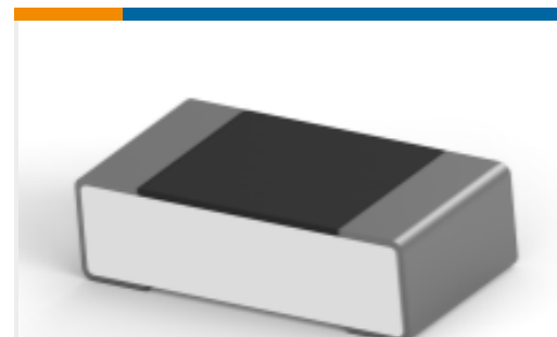
TE Part #2176368-3 RQ 0603 52K3 0.1% 10PPM 1K RL
