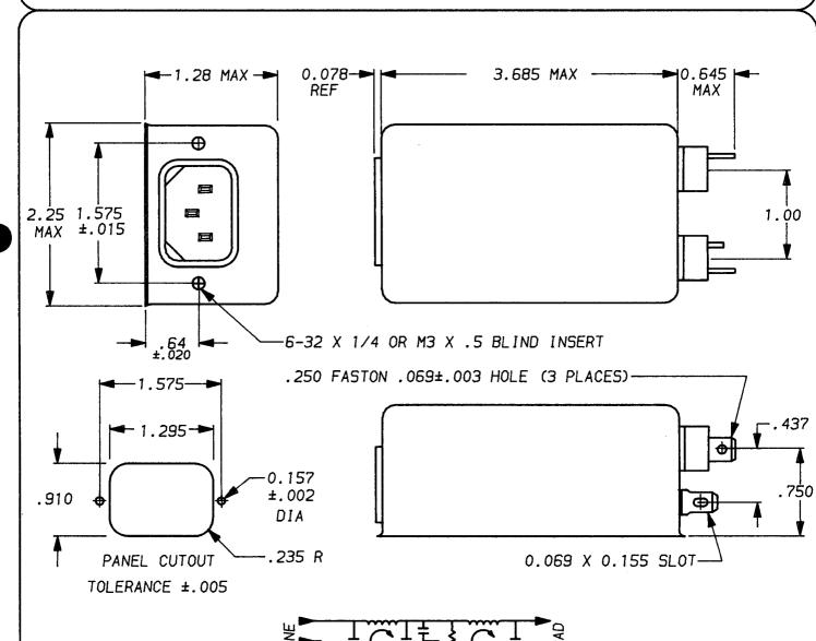
UNLESS OTHERWISE SPECIFIED, (MINIMUM) INSERTION LOSS TOLERANCE TO BE ±.025 FREQUENCY . 15 .3 .5 2 10 20 30 MHz MATERIAL & FINISH: AS SUPPLIED POWER LINE FILTER COMMON This document is proprietary to CORCOM INC. and is not to be reproduced nor used for manufacturing purposes except on CORCOM'S prior written consent. 30 50 65 65 65 65 65 65 ď₿ DATE: 9-16-93 CATALOS NO. DIFF APPRIOR TO MINISTRA & 3VR7M 65 50 65 65 65 65 65 3VR7.08
