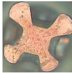
Uneven Crimp and Wall Thickness
