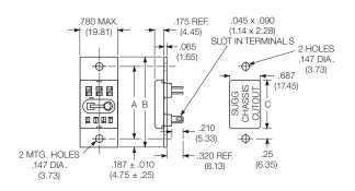
Track mount sockets 27E460, 27E461, 27E462 Provides front wiring, screw terminal connections for R10 family relays. No grounding provision.
