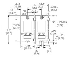
24A110 – Mounting track Mounting track is designed to accept snap-mount sockets, as well as other P&B screw terminal sockets. Track is made of lightweight, sturdy extruded aluminum and is shipped in three-foot (914cm) lengths with mounting holes on six-inch (152mm) centers. Track can be cut to shorter lengths or used end-to-end.
