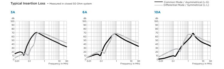
Minimum Insertion Loss - Measured in closed 50 Ohm system
