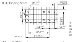
\*) With the recommended PCB hole sizes a grid pattern from 2.5mm to 2.54mm can be used.
