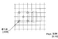
Recommended Mounting holes for Part No. 1-1393662-2 and 1-1393662-4
