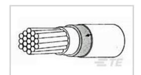
Cable Type: Spec 55F Voltage Rating: 600 V
