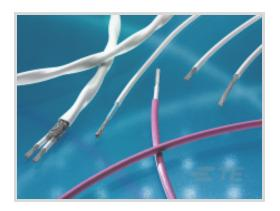
Cable Type: Spec 55 Voltage Rating: 600 V Insulation Material: Modified Radiation Cross-linked ETFE Polymer Conductor Material: Tin-Coated Copper Wire Size: 16 AWG
