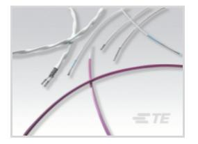
Twisted Pair Cable Type: Spec 55 Twisted Pair Cable Voltage Rating: 600 VAC Twisted Pair Cable Insulation Material: Modified Radiation Cross-linked ETFE Polymer Twisted Pair Cable Conductor Material: Tin-Coated Copper Wire Size: 14 AWG
