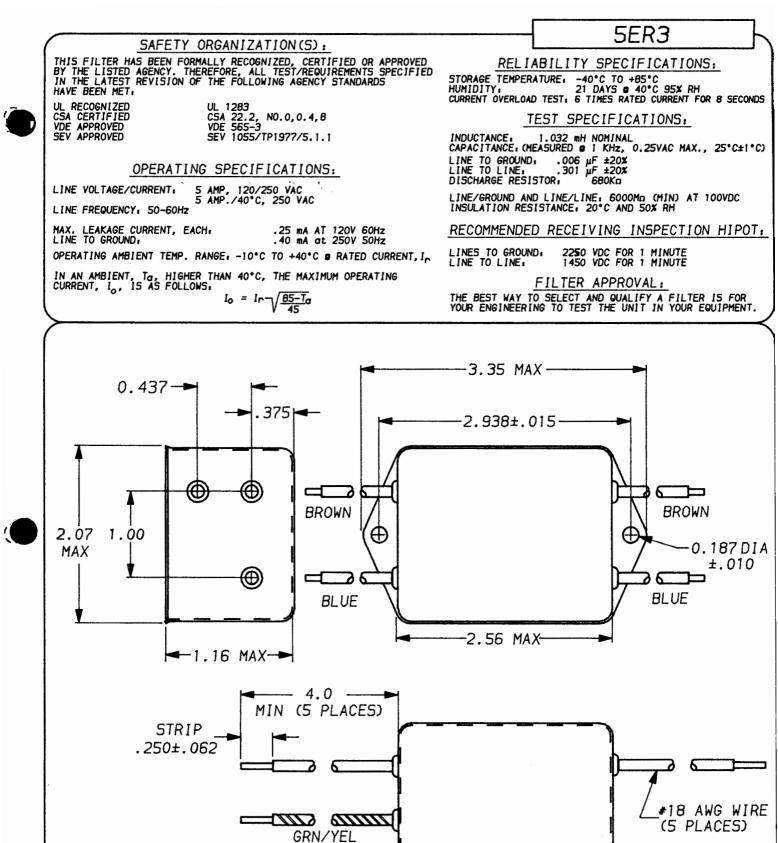
UNLESS OTHERWISE SPECIFIED, 50n - 50n (MINIMUM) INSERTION LOSS TOLERANCE TO BE ±.025 . 15 .5 1 2 5 10 20 30 MHz MATERIAL & FINISH: AS SUPPLIED POWER LINE FILTER COMMON This document is proprietary to CORCOM INC. and is not to be reproduced nor used for manufacturing purposes except on CORCOM'S prior written consent. 2 33 41 57 65 65 65 65 65 dΒ DATE: 9-24-93 CATALOG NO. DIFF 3 3 19 CAD NO. 5ER3 ď₿ 5ER3.04
