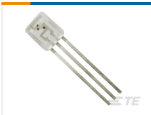
TE Part #11032254-00 EMITTER 660/940NM 1 2
