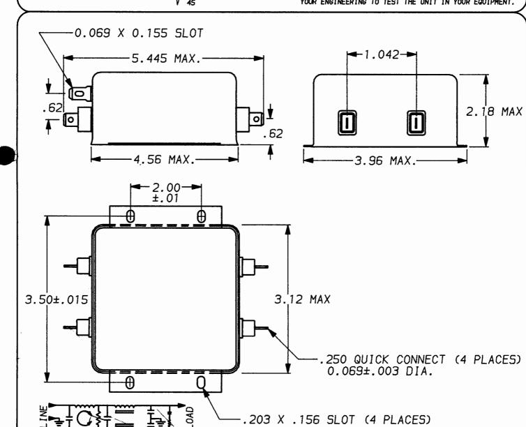
UNLESS OTHERWISE SPECIFIED, TOLERANCE TO BE ±.025 50a - 50a (MINIMUM) INSERTION LOSS . 15 .03 .05 .07 .1 .З .5 5 10 20 30 MH2 MATERIAL & FINISH: AS SUPPLIED COMMON This document is proprietary to CORCOM INC. and is not to be reproduced nor used for manufacturing purposes except on CORCOM'S prior written consent. POWER LINE FILTER 8 22 25 29 33 45 44 52 52 57 35 ď₿ DATE: 9-28-93 CATALOS NO. DIFF APPRIO. THE M 19 15 13 70 70 70 70 65 60 15VT1 dΒ CAD NO. 15VT1.07
