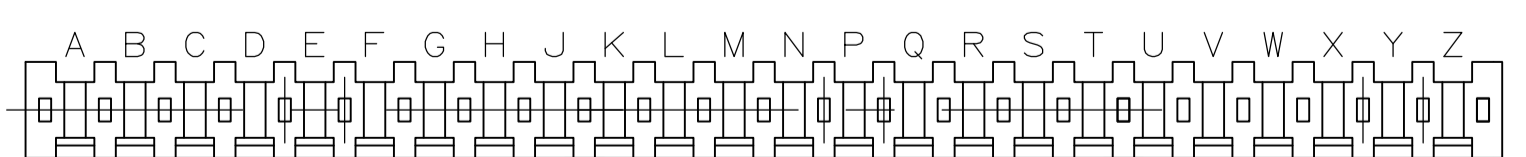
KEYWAY LOCATIONS (REF-SEE TABLE) (MATING LENGTH OF POST ON NEAR SIDE) SCALE: 2:1
