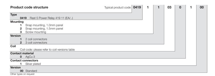
**Product code** Cont. material Version Cont.arrangement Coil Part number 0419 11 0301 00 Snap Mounting AgCu3 2 form A, 3-1415419-5 AC coil 4-1415419-0 0419 11 1201 00 1.0mm plate 2 NO DC coil 0419 11 1301 00 contacts 4-1415419-2
