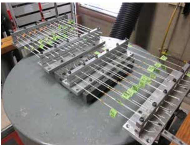
Figure 2 – Military Vibration Test - SOLISTRAND Splices
