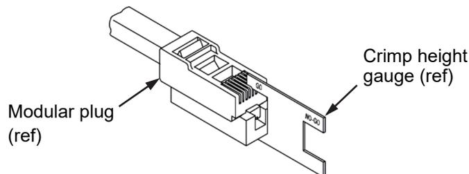
**Figure 4. Crimp Height Gauge**
