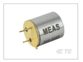
Acceleration Range (±): 50 g Frequency Response: 1 to 8000 Hz Accelerometer Type: 3-Wire Voltage Number of Axes: 1 Sensitivity: 40 mV/g
