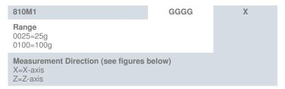
Examples; 810M1-0025X Model 810M1, 25g range, X-axis measurement
