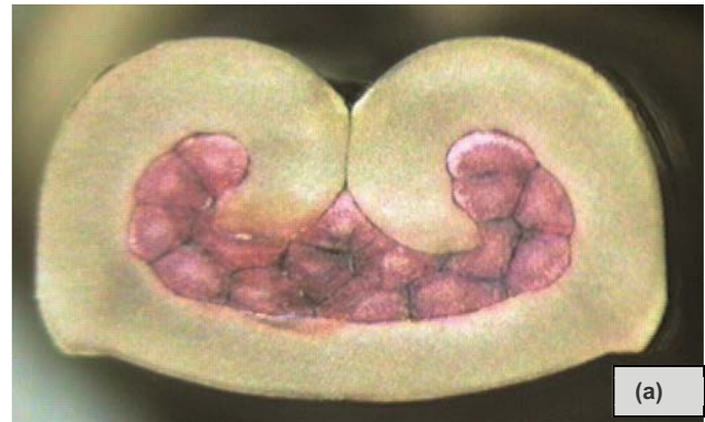
Cross Sections Showing Minimum (a) and Maximum (b) Area Index per Terminal Specification—a Variation of \pm 3.5\%
