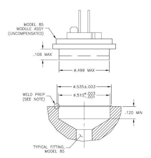
NOTE: WELD PREP SHOWN IS FOR RESISTANCE WELD. ACTUAL GEOMETERY VARIES PER CUSTOMER REQUIREMENTS.
