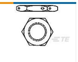
TE Part #2-332004-0 SMA JAM NUT, PASSIVATED
