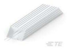
The CJH Series of resistors are an economical and compact aluminium housed resistor with good electrical stability and reliability. With power ratings up to 5000W they are suited to a range of electrical circuits including power supplies inverters and servo systems. With very good durability and mineral filled construction they are particularly good for braking and other pulse applications.
