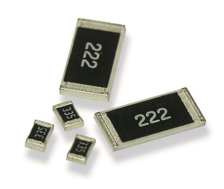
The resistive element is screen printed and fired, and a passivation layer added. Each resistor is trimmed to tolerance by laser. The pre-scribed tile is then broke into strips, the end plating fired on, and the strips broken into individual components. Final termination finish is electroplated matte Sn over a Ni barrier layer.
