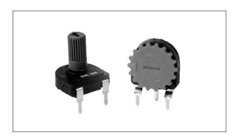
Low price, versatility and stable environmental characteristics are important benefits of this product. Featuring an innovative carbon resistive element printed on film in a fully enclosed package, this potentiometer style is normally chosen for a wide range of applications in industrial, professional and consumer equipment.
