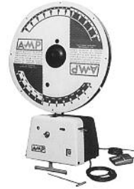
AMP-TAPEMATIC Stripper/Crimper Machine Part Number 599406-7 Funnel Part Number 125905-1 for Size 20 Contacts
