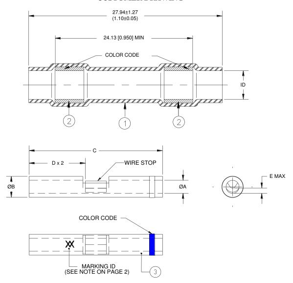
\* I.D.: a) As received; b) After unrestricted recovery thru meltable insert.
