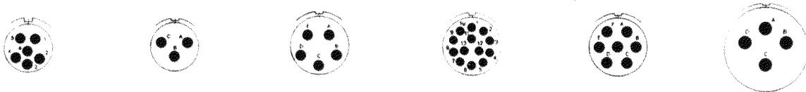
09-35 6 SIZE 220 CONTACTS 09-98 3 SIZE 20 CONTACTS 11-05 5 SIZE 20 CONTACTS 11-35 13 SIZE 220 CONTACTS 11-99 7 SIZE 20 CONTACTS 13-04 4 SIZE 16 CONTACTS
