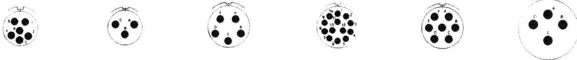
09-35 6 SIZE 220 CONTACTS 09-98 3 SIZE 20 CONTACTS 11-05 5 SIZE 20 CONTACTS 11-35 13 SIZE 220 CONTACTS 11-99 7 SIZE 20 CONTACTS 13-04 4 SIZE 16 CONTACTS
