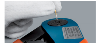
STEP 3: Insert the contact in the crimping tool.
