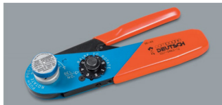
STEP 1: Use a crimping tool with the appropriate locator.
