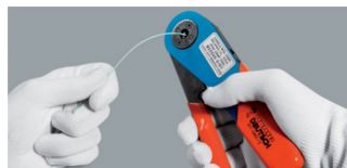
STEP 5: Tighten the crimping tool.
