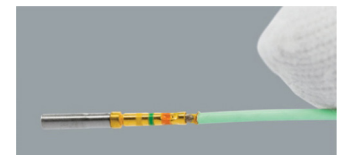
STEP 6: Inspect the contact. It must have 8 indents, and the wire must be seen in the contact inspection hole.
