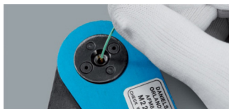
STEP 4: Insert the wire in the contact.
