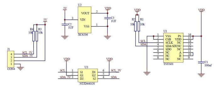
Connector Pin Assignments (I<sup>2</sup>C Communications)
