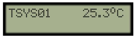
Sensor measurements are refreshed every 500 milliseconds.
