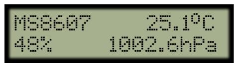
Sensor measurements are refreshed every 500 milliseconds.
