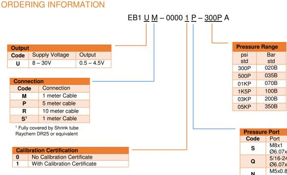
The **psi** range models are only supplied with imperial thread design. The **bar** range models are only supplied with metric thread design
