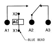
**NOTE:** Polarity must be observed with DC coil supply. Relay is polarized with a permanent magnet and will not operate or be damaged by reverse polarity.
