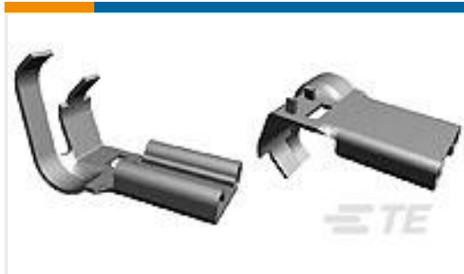
TE Part #63517-1 250 FLG FAST REC 18-12 TPBR
