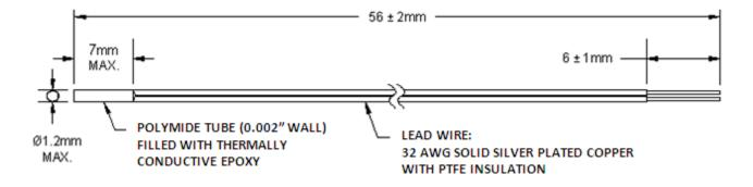
Figure 1: Mini BetaCURVE Thermistor Probe (MRBD) - High Humidity environments
