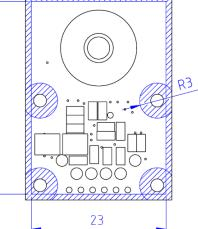
Only use hatched areas for mechanical assembly (screws, nuts, etc).
