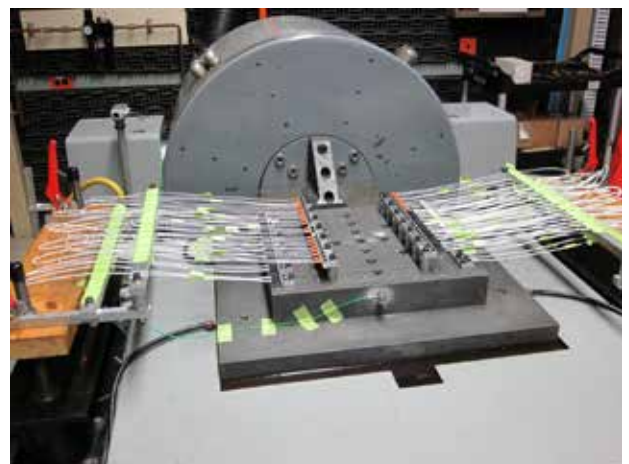
Figure 3 – Military Vibration Test - PIDG Terminals
